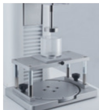
EXTRUSION FIXTURE (Ref. 100200)
