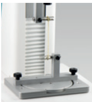
NOODLE TENSILE FIXTURE (Ref. 130168)
